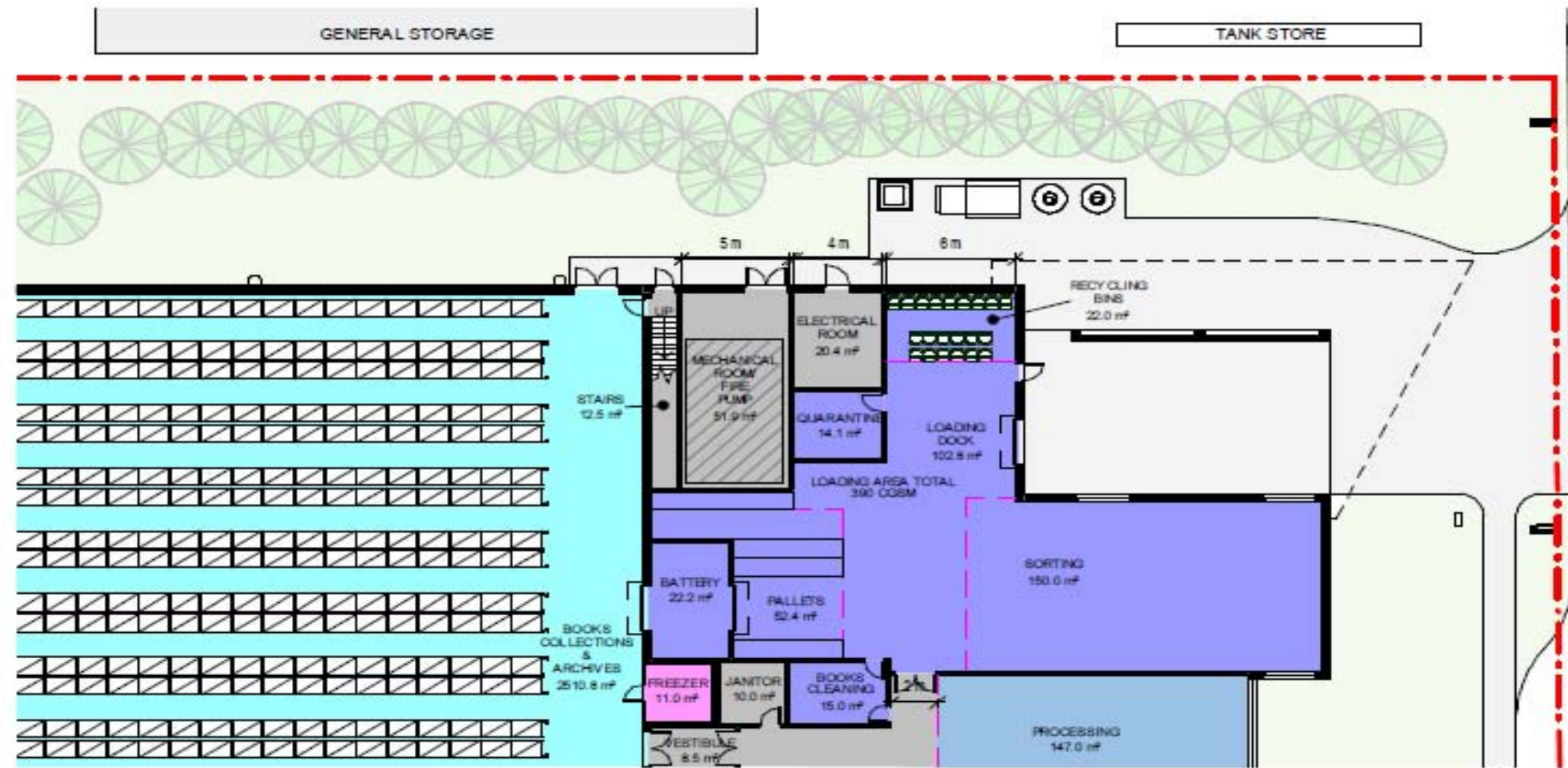
Partial Plan - Spatial Separation & Exposure Protection (not to scale)
