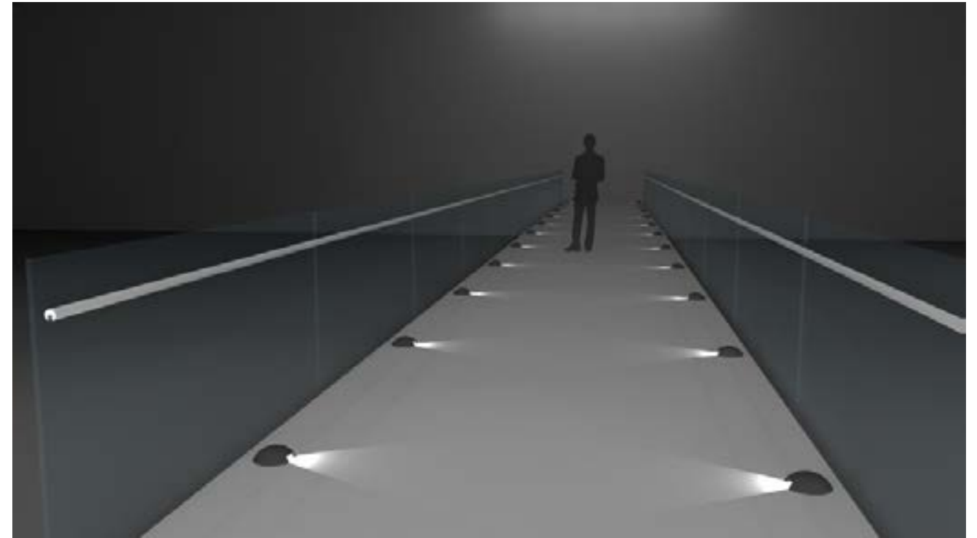
Figure 7 Typical Atrium Bridge Lighting
