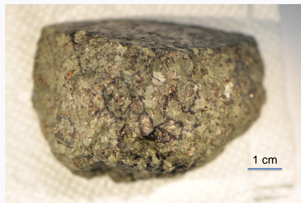
Figure 2. (left) Map of southern Africa detailing the occurrence of major kimberlite pipes within the Kalahari craton (2). Figure 3. (right) Visible light image of the RV09 sample. One half underwent jaw crushing while the other half went into the SELFRAG.
