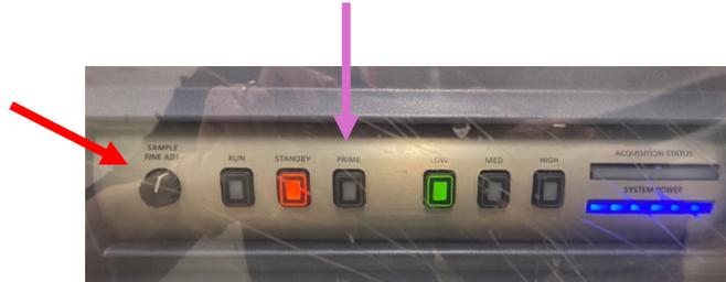
Do not touch the Sample Fine Adj knob (red arrow). Only modify acquisition speed using Low, Med and High buttons.
