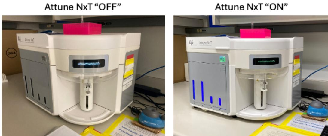
1. Ensure instrument's Focusing fluid, Wash and Shutdown containers are full, and that waste is empty
