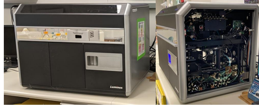
Cytek Amnis ImageStream mkII Imaging Flow Cytometer – combines imaging and flow cytometry
