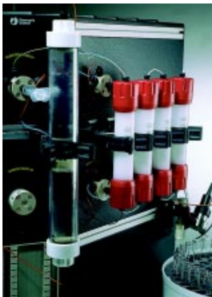
Fig. 10. Four HiPrep 26/10 Desalting columns connected in series.
